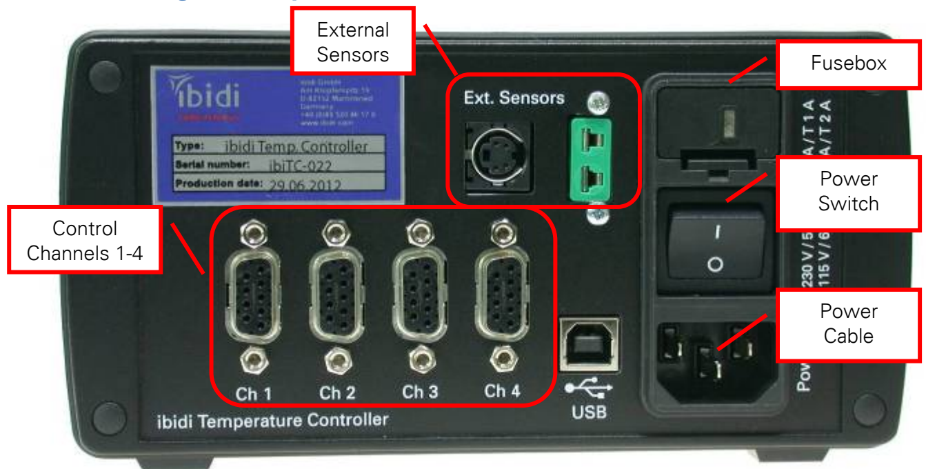
Figure 3: Rear Panel of the ibidi Temperature Controller
