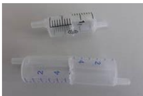
Figure 4 Example of a simple DIY bubble trap.
